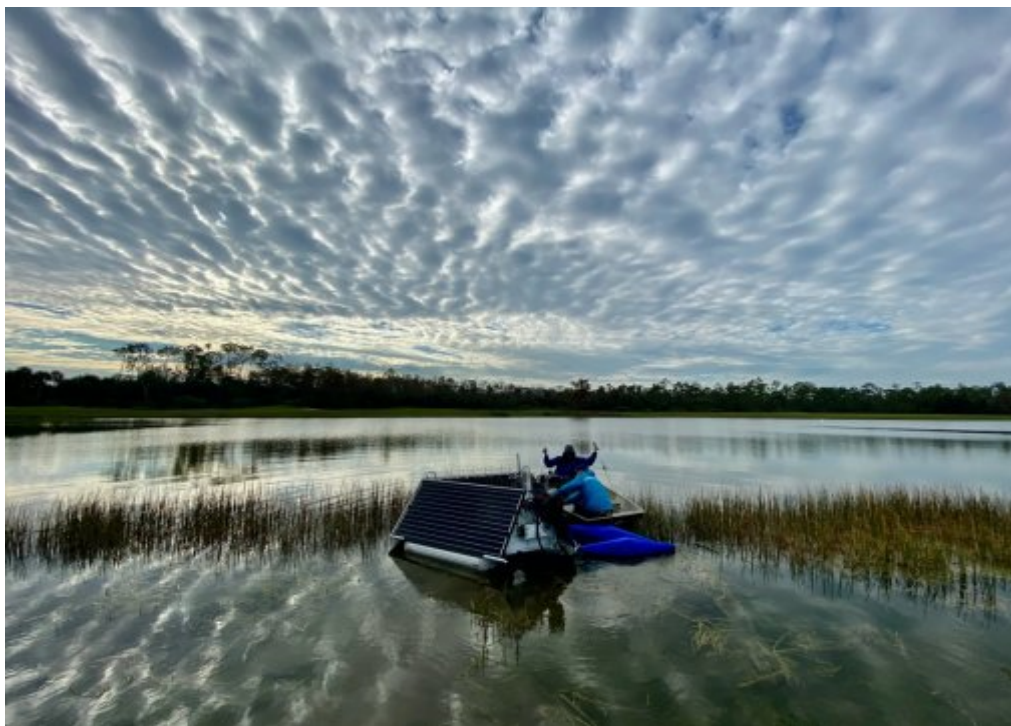
Figure 3. Deployed sonic buoy in one of the experimental lakes at Treviso Bay.
