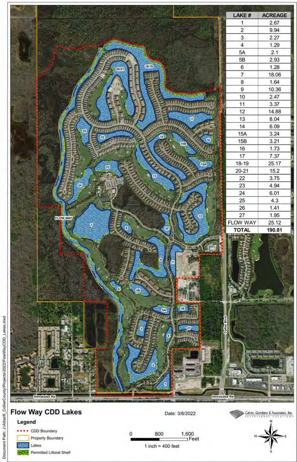
Figure 5-1. Flow Way CDD Lakes Map, showing all 27 lake systems and the Flow Way water body with corresponding acreage (190.81 total acres), the CDD and property boundaries, and areas of permitted littoral shelf. This map identifies which lake banks currently lack established littoral shelf coverage and should be prioritized for the planting and maintenance work described in this chapter and in Chapter 3. Date: 3/8/2022, Calvin, Giordano & Associates, Inc.
