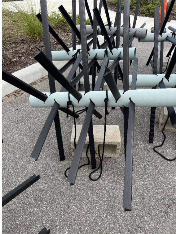
Structure with attached block for anchorage.
